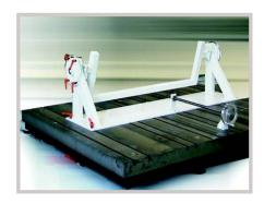
An adjustable instrument panel test stand is used for mounting the instrument panel or other test specimen. It is adjustable longitudinally (e.g. on a T-slot base plate) as well as rotating the IP along around the Y-axis.
