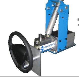
When tuned for cover testing, the CGS output pressure curve closely follows the pyrotechnic inflator curve during the initial 20msec. The corresponding high speed video demonstrates the accuracy of the CGS as a pyro replacement.
